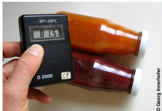
Hot filling is the best known method for the preservation of non-sparkling (devoid of carbon dioxide) drinks. It is employed at temperatures, lower than 100 °C and therefore is known as one method, known as pasteurization. Bacteria, which later could cause spoilage, are eliminated by means of heat.
