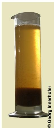
Even under highest technical standards, flaky residues and lump formation at the bottle's bottom can't be completely eliminated.
