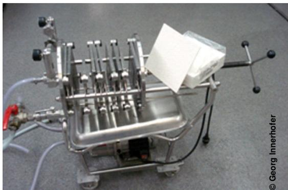
In most cases, cosmetic treatment on its own is not sufficient, in order to maintain clear or bright juice qualities. Thus, all cosmetic treatment is normally flanked by a filtration process and finally completed by heat treatment and bottling. In general, hot-filling following diatomite filtration will make sterilisation obsolete.
